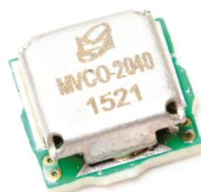
MVCO-2040-F is an octave VCO that can be used in wideband PLL synthesizers for telecommunications and T&M equipment. High-quality components and careful design guarantees repeatability of parameters, high reliability and low cost at mass production stage.
